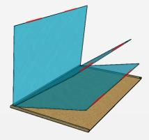
**Step 5** - Lift the glass from its now exposed edge, supporting the glass in multiple places along the edge to bring the glass upright while being careful to prevent excessive flexing or bowing of the glass.
